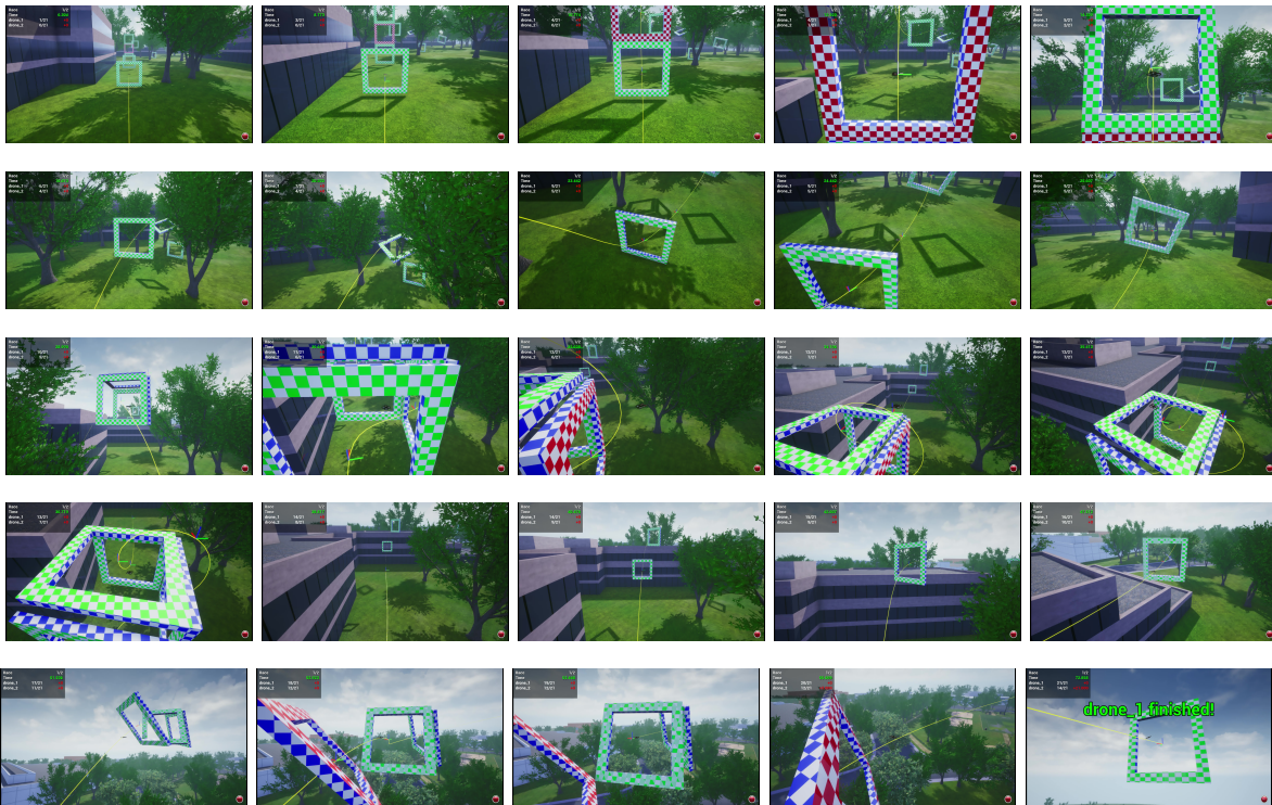
Fig. 1. Examples of the best run. The speed and acceleration used for Gate 1 to 19 is 106 m/s and 28.7 m/s respectively, and for Gate 20 to 21 it is 27 m/s and 21 m/s.
