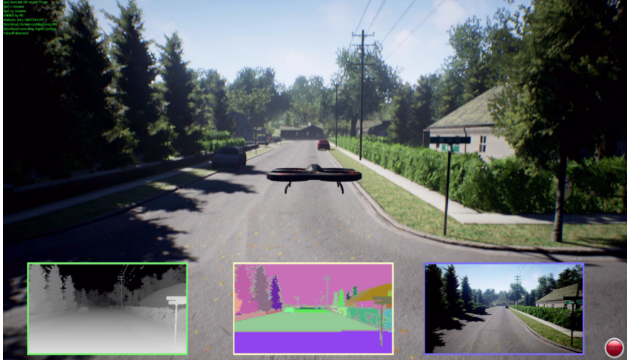
Fig. 1 A snapshot from AirSim shows an aerial vehicle flying in an urban environment. The inset shows depth, object segmentation and front camera streams generated in real time.
